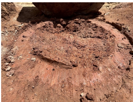
Figure 5. 300 kPa strong alteration saturated shear surface
