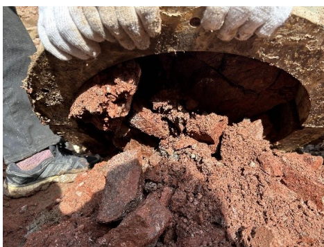
Figure 4. 300 kPa strong alteration natural shear surface
