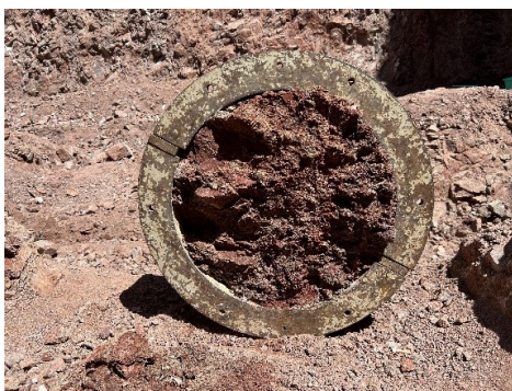
Figure 2. 200 kPa weak alteration natural shear surface
