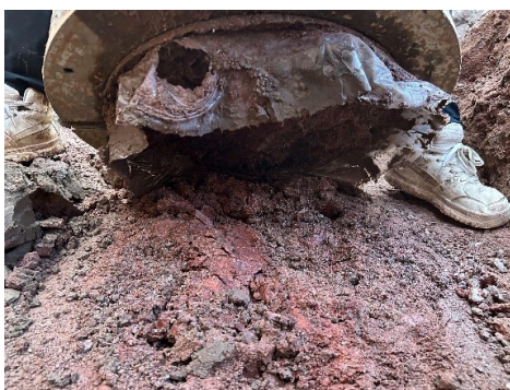
Figure 3. 300 kPa weak alteration saturated shear surface
