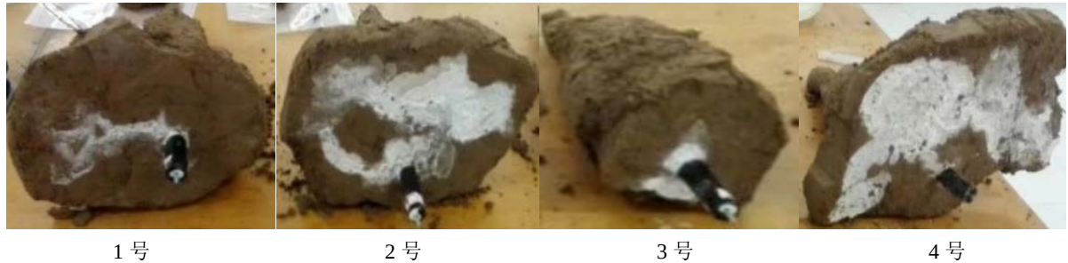
Figure 6. Diffusion radius of each grouting pipe surface
