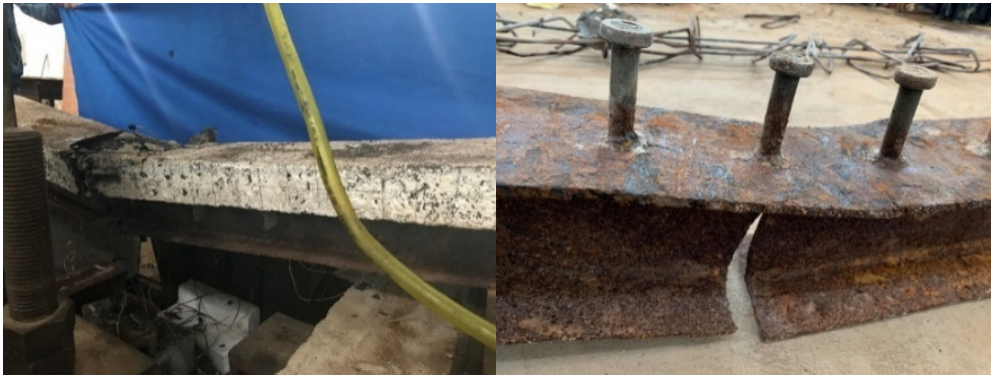
Figure 6. Fatigue failure mode 图 6. 试件疲劳破坏形态
