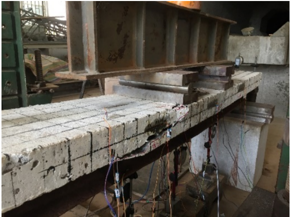
Figure 5. Static failure mode of composite beams 图 5. 组合梁静力破坏形态
