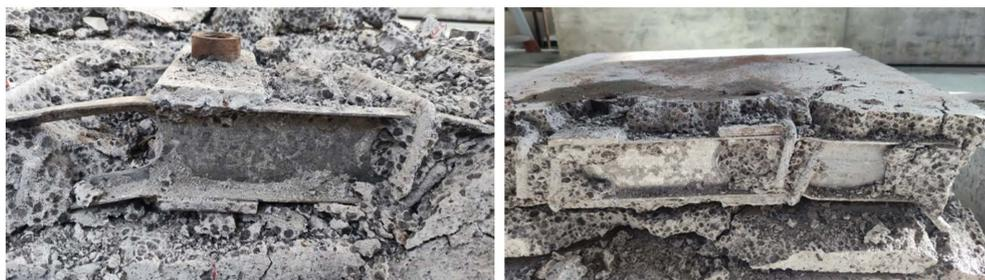
**Figure 4.** Keel steel frame and steel reinforcement deformation of typical specimens
