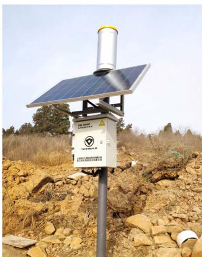
Figure 6. Tipping bucket rain gauge
