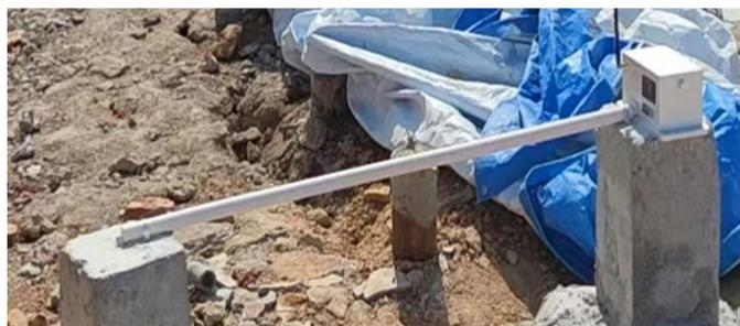
Figure 5. Pull rope crack meter
