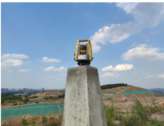
Figure 2. Monitoring robot
