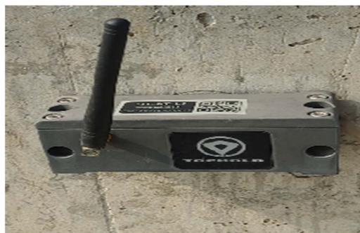
Figure 4. Wireless collapse meter
