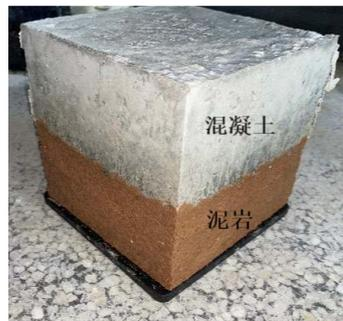
**Figure 2.** Sample after release curing
