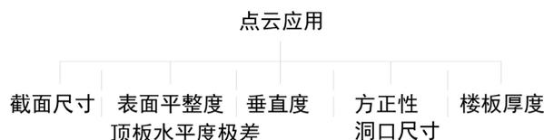
Figure 2. Point cloud application classification of measured real indicators
