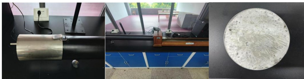
Figure 2. Sound absorption coefficient measuring instrument for standing wave tube (left, center); Sample test block (right) 图 2. 驻波管吸声系数测量仪(左、中); 试块样例(右)
