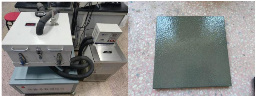
Figure 1. Double flat plate thermal conductivity tester (left); Sample test block (right) 图 1. 双平板导热系数测定仪(左); 试块样例(右)
