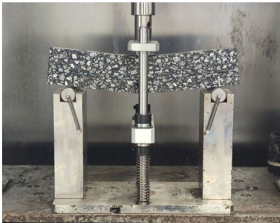
Figure 3. Bending test of small beam 图 3. 小梁弯曲试验
