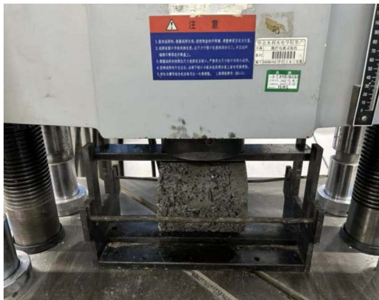
Figure 3. Splitting strength test 图 3. 劈裂强度试验
