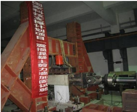
Figure 5. Installation of test pieces 图 5. 试件安装情况图
