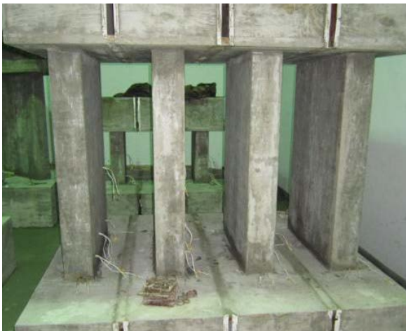
Figure 4. Photograph of test piece molding 图 4. 试件成型照片
