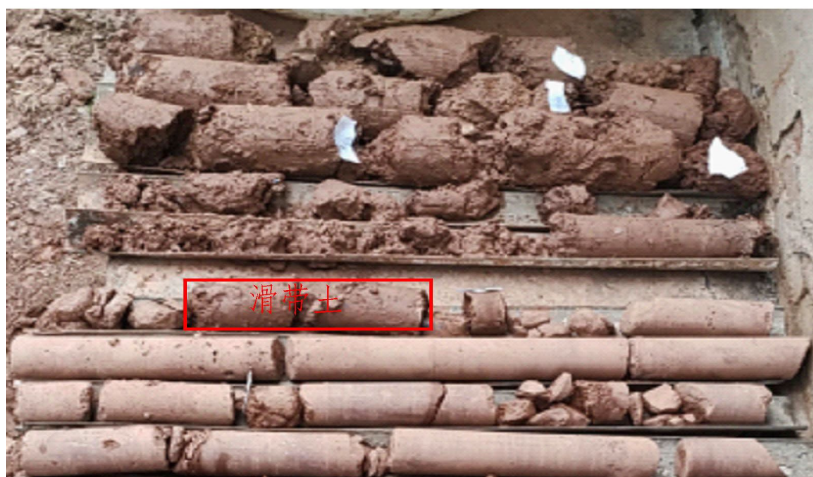
Figure 9. Drill holes to expose slip-zone soils 图 9. 钻孔揭露滑带土
