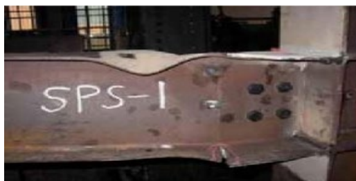
Figure 2. Reinforcement of flange side plates with dog-bone failure pattern 图 2. 翼缘侧板加固狗骨式破坏形态
