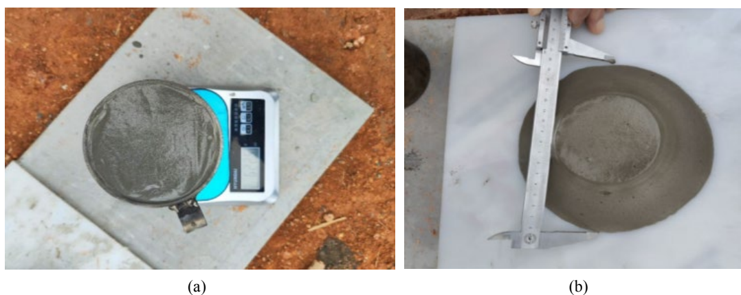
Figure 17. On-site quality inspection of foam lightweight concrete
