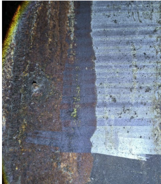
Figure 2. Laser rust removal effect on steel structures 图 2. 钢结构激光除锈效果
