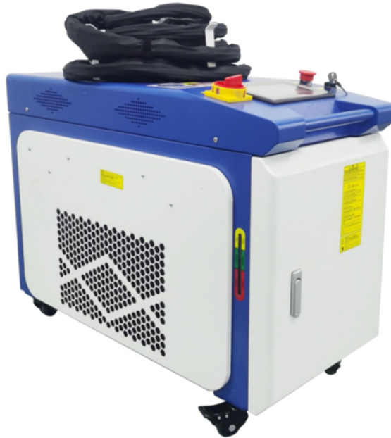
Figure 1. Laser rust removal equipment for steel structures 图 1. 钢结构激光除锈设备
