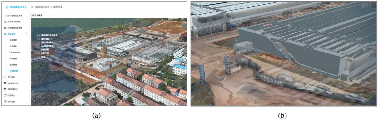
Figure 3. Integration of 3D reality model with BIM model. (a) Digital twin platform convergence diagram; (b) Partial diagram of model integration
