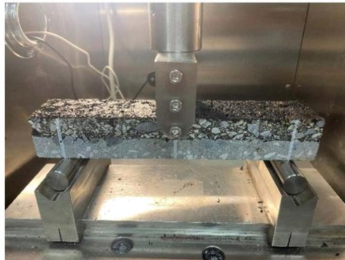
Figure 2. Composite specimen test device
