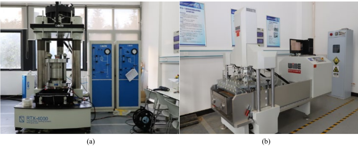
Figure 2. Large-scale indoor testing apparatus: (a) Rock triaxial testing machine (b) Rock direct shear testing system 图 2. 室内大型试验装置：(a) 岩石三轴试验仪(b) 岩石直剪试验系统
