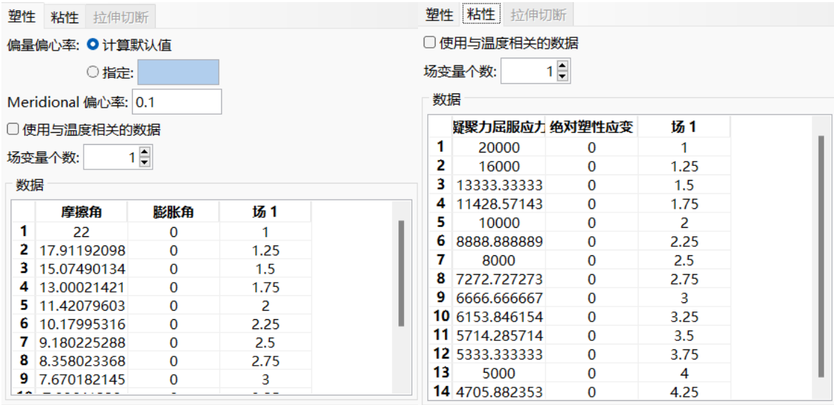
Figure 2. Reduction of shear-strength parameters c and \varphi with field-variable evolution 图 2. 抗剪强度指标 c 、 \varphi 值随场变量变化折减
