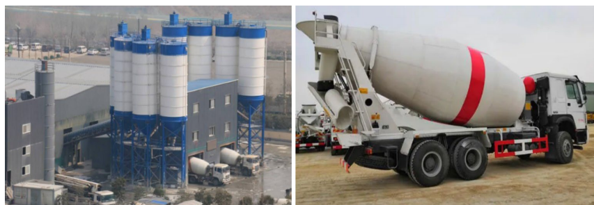
Figure 3. Concrete mixing and transportation 图 3. 混凝土搅拌与运输
