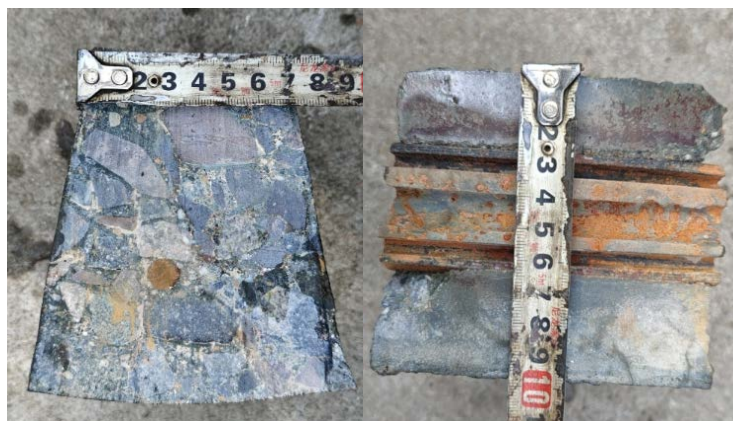
Figure 10. Minimum particle size measurement
