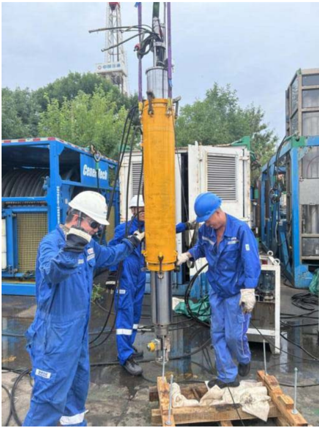
Figure 4. Improved design of the high-pressure jet nozzle 图 4. 高压射流喷头改进设计
