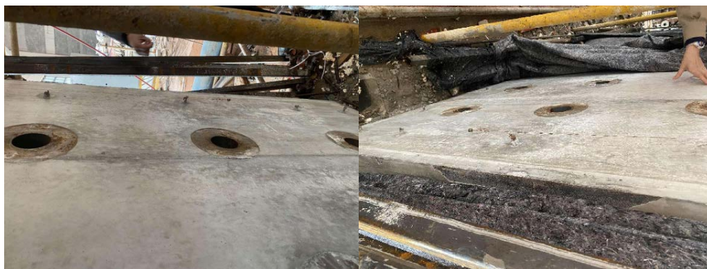
Figure 8. Overall appearance of fully recycled coarse aggregate concrete 图 8. 全再生粗骨料混凝土表现
