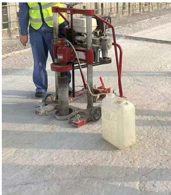
Figure 4. Core sample testing
