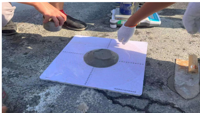
Figure 2. On-site testing of the fluidity of foamed concrete
