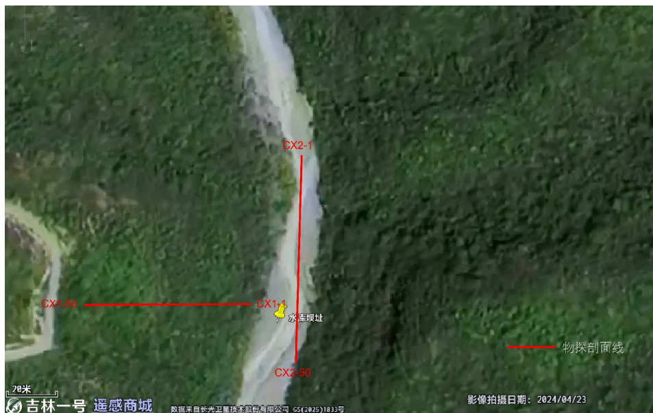
Figure 4. Location map of high-density electrical method survey lines 图 4. 高密度电法测线位置图
