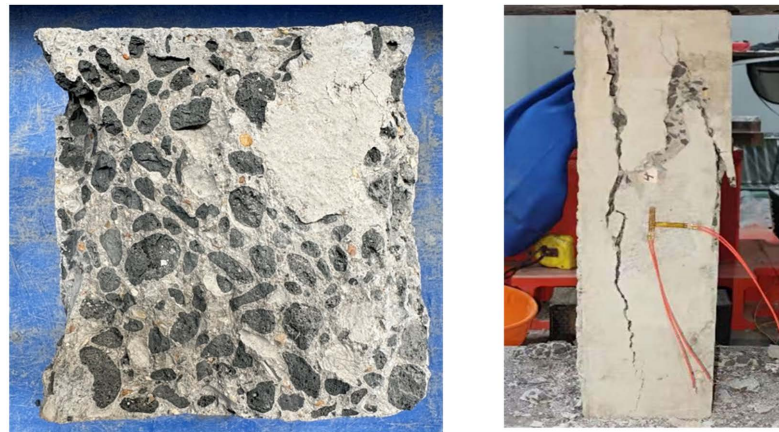
Figure 2. Material property testing of ceramsite concrete 图 2. 陶粒混凝土材性测试
