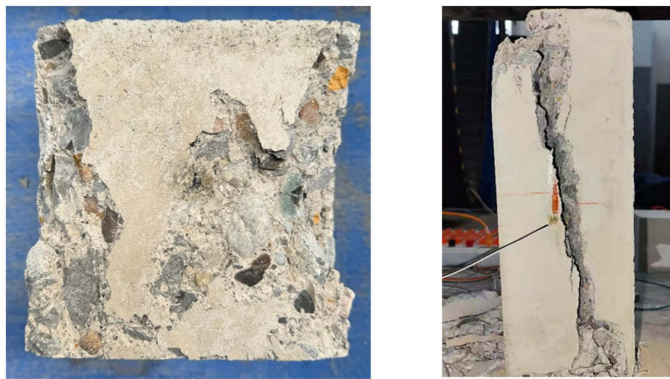
Figure 1. Material property testing of normal concrete 图 1. 普通混凝土材性测试
