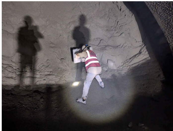
Figure 2. On-site GPR testing image
