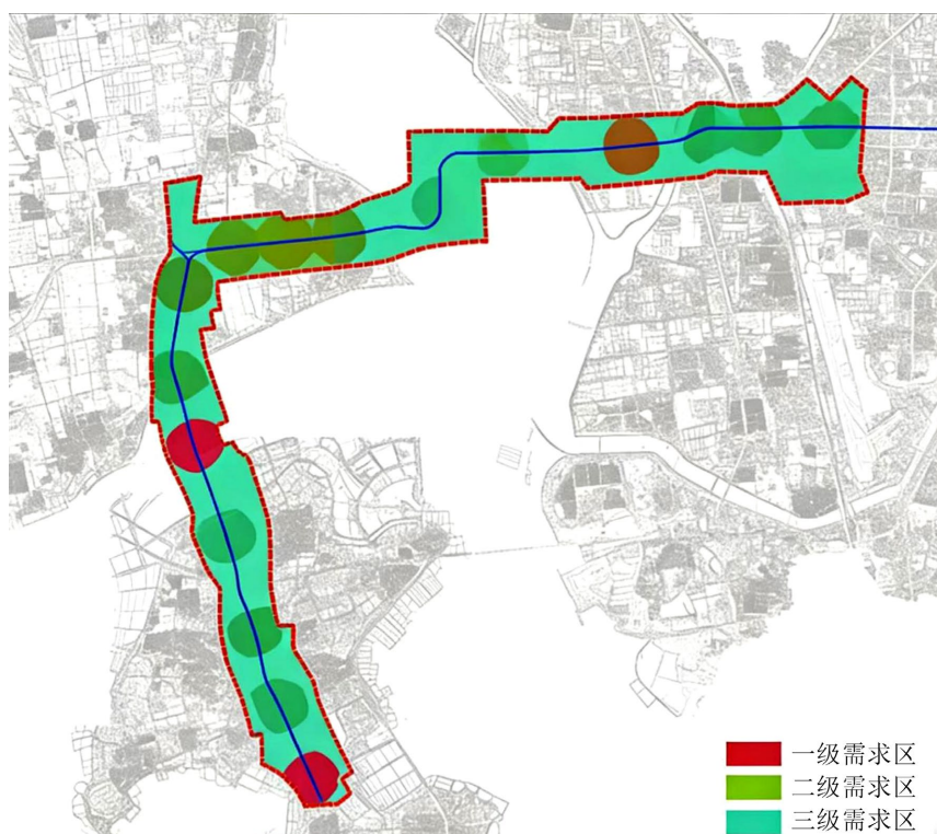
Figure 4. Schematic of demand assessment results along subway lines 图 4. 地铁沿线需求评估结果示意图
