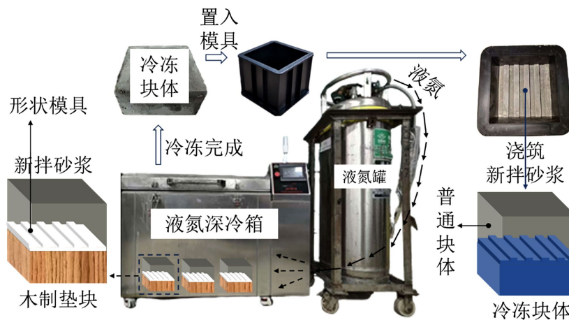
Figure 1. Casting process of composite specimens
