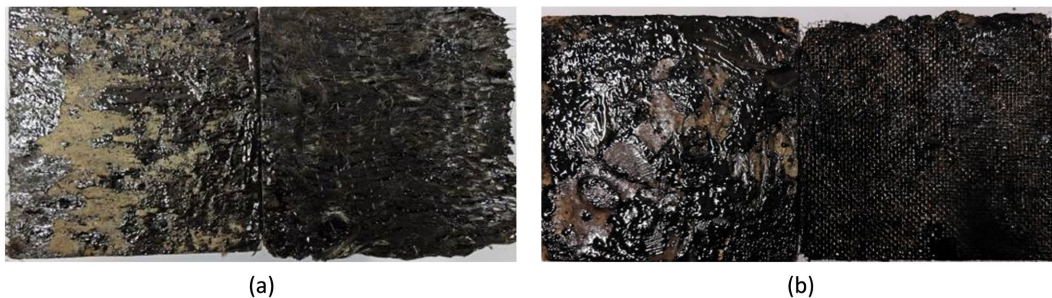
Figure 6. Interlayer interface morphology. (a) Basalt fiber fabric; (b) Steel wire mesh 图 6. 层间界面形态。(a) 玄武岩纤维布；(b) 钢丝网
