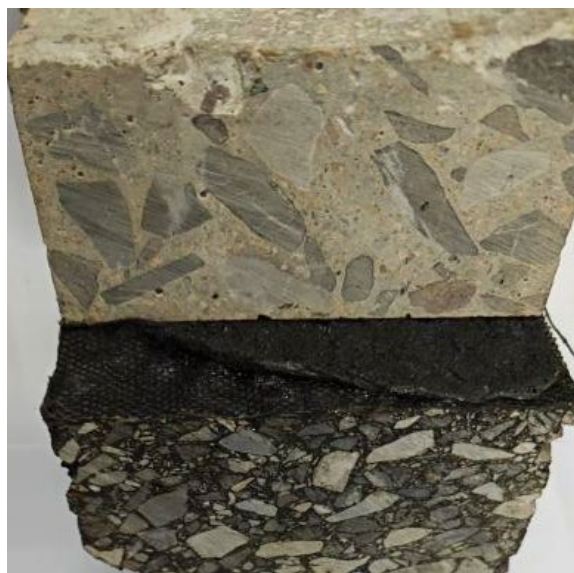
Figure 7. Shear morphology of the composite specimen with stress-absorbing membrane 图 7. 应力吸收贴复合试件剪切形态
