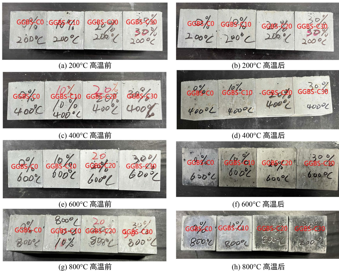
Figure 2. Appearance before and after high-temperature treatment 图 2. 高温前后外观形貌
