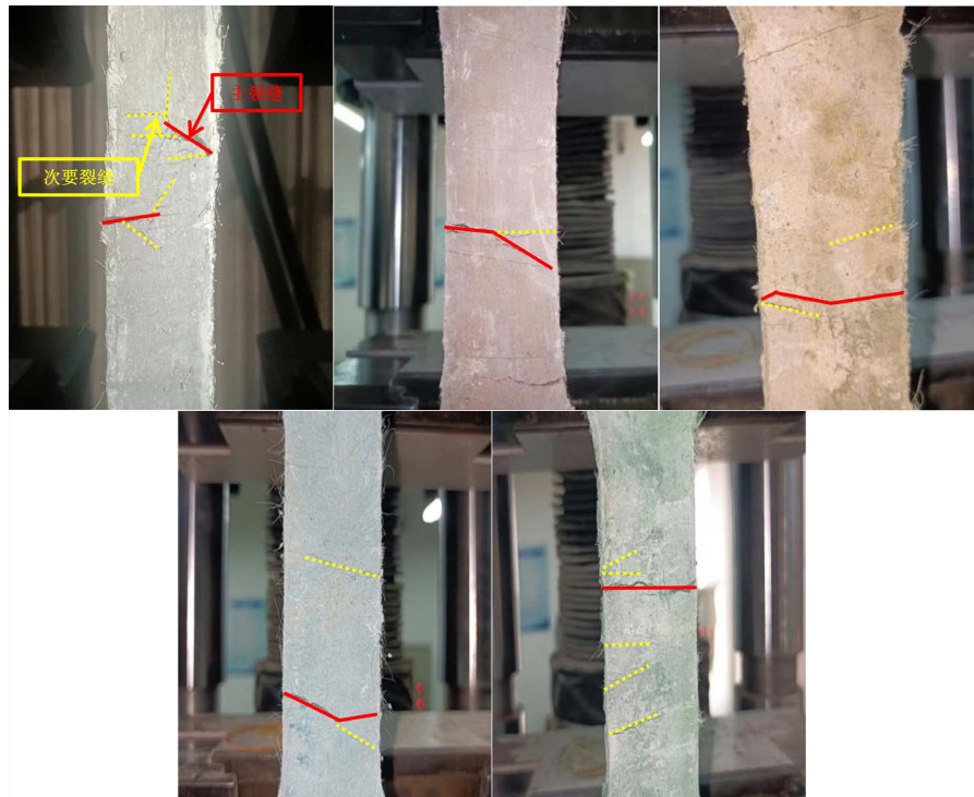
Figure 6. Cracks in normal ECC dumbbell specimens and colored ECC specimen sections
