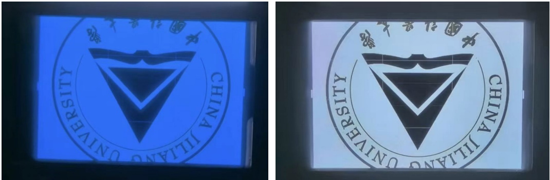
Figure 1. Photograph showing electrochromic effect of smart glass (Left: Colored state; Right: transparent state) 图 1. 智能玻璃电致变色效果实物展示图(左：着色态；右：透明态)
