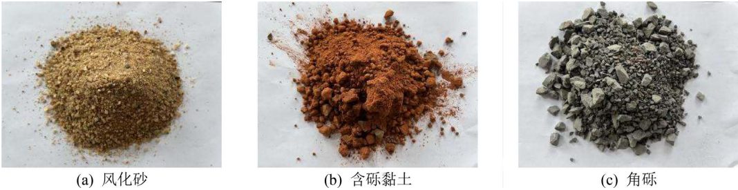
Figure 1. Soil samples with different fillers 图 1. 不同填料土样
