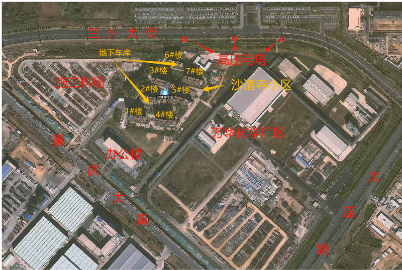
Figure 1. Buildings for blasting demolition and surroundings 图 1. 待爆破楼房
