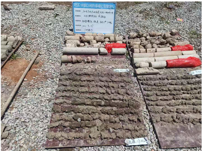
Figure 1. Insufficient pile length 图 1. 桩长不足
