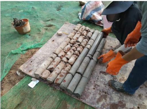
Figure 4. Core-drilling photograph of cement mixing pile after implementation of optimal countermeasures 图 4. 最优对策实施后水泥搅拌桩取芯图
