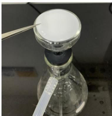
Figure 1. Filter mounting
