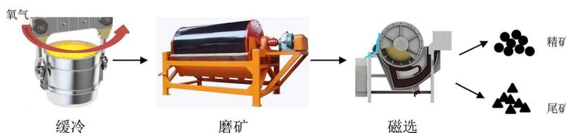
**Figure 5.** Schematic diagram of selective oxidation-magnetic separation of copper slag
