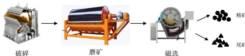
**Figure 4.** Schematic diagram of direct magnetic separation of copper slag
