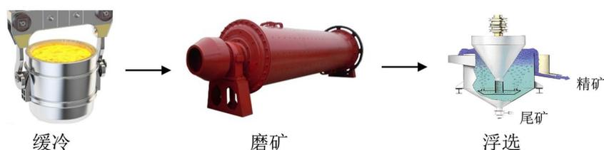
Figure 2. Schematic diagram of slow cooling-flotation of copper slag
