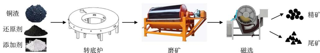
Figure 6. Schematic diagram of direct reduction-magnetic separation of copper slag
