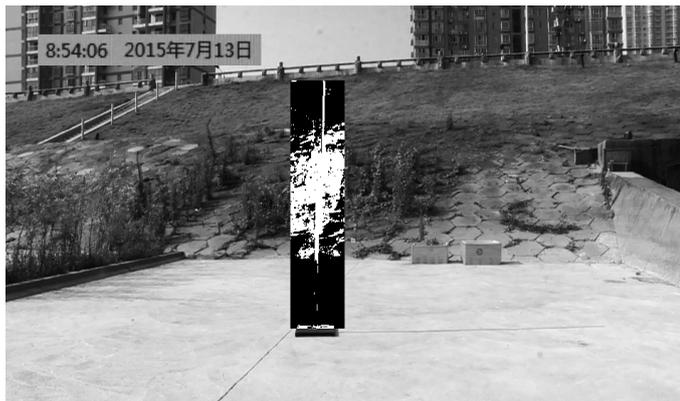
**Figure 5.** Gray level images after binarization of straight rod matrix
