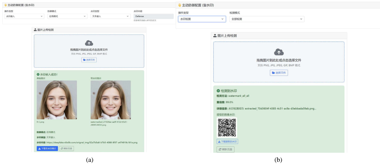
Figure 3. Blind watermark embedding/detection: (a) Example of online text watermark embedding; (b) Example of online QR code watermark extraction
