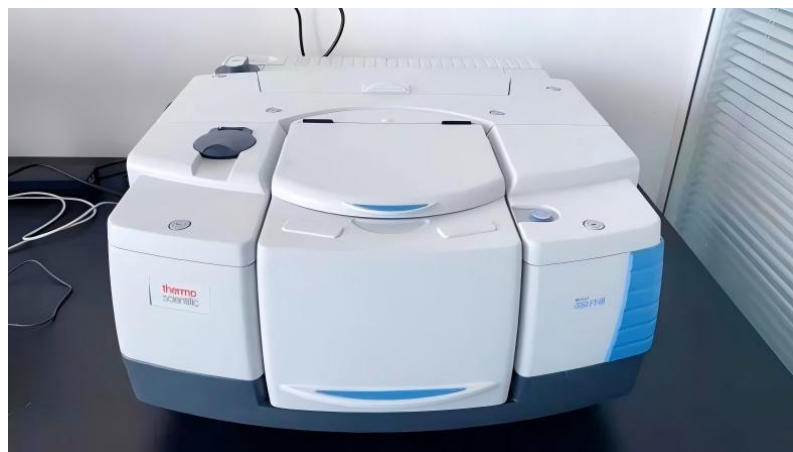
Figure 3. BFH-960 Fourier transform infrared spectrometer GBPI 图 3. BFH-960-傅立叶变换红外光谱仪 GBPI
