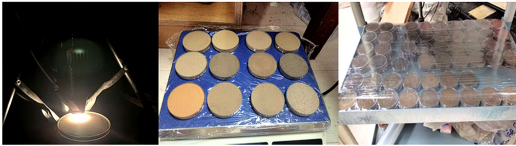
Figure 2. Laboratory spectral measurements of dry and wet soils 图 2. 干土与湿土实验室光谱测量
