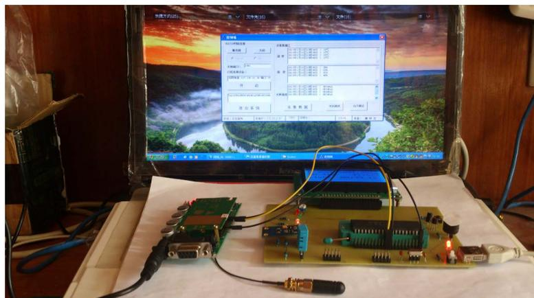
Figure 15. GPRS transferring data test
