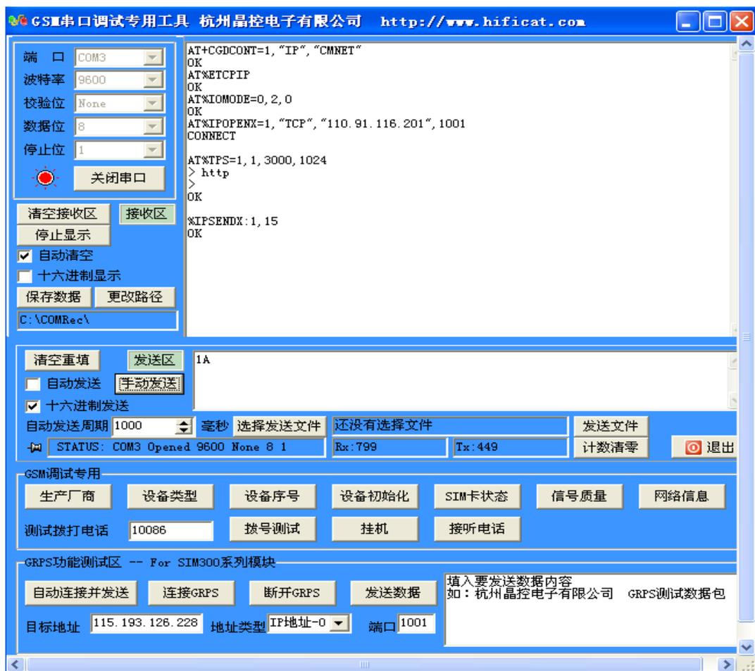
Figure 9. GPRS Networking test serial debugging assistant figure
