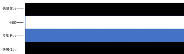
**Figure 6.** “Sandwich” shielding jacket isolation prototype
