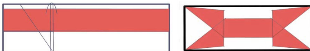
Figure 3. Lap area of heat sealing BOPP film of small cigarette package
