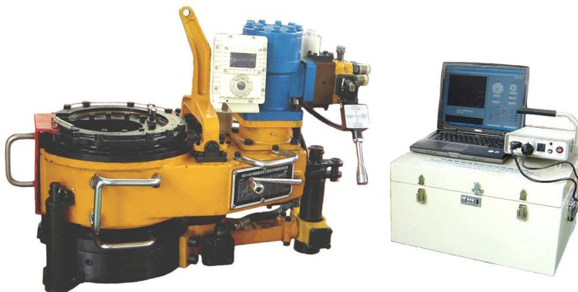
Figure 5. Real picture of torque monitoring system
