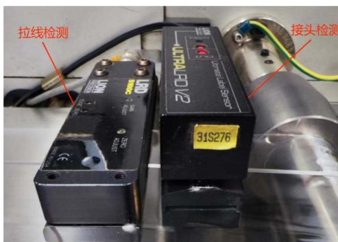
Figure 4. LRD5100C tear-tape detection and ULTRA LRD V2 transparent paper splice detection
