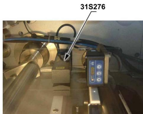
**Figure 2.** Detection of transparent paper splice using ULTRA LRD V2
