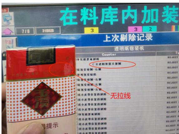
Figure 7. The rejection effect of LRD5100C tear-tape detection
