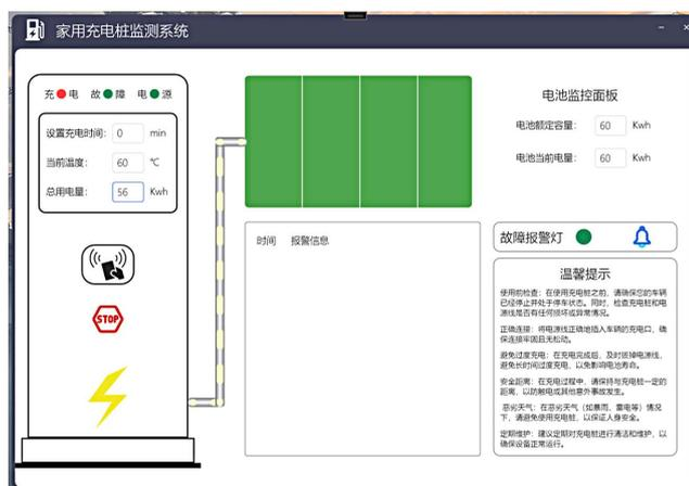
Figure 9. Normal operation interface
