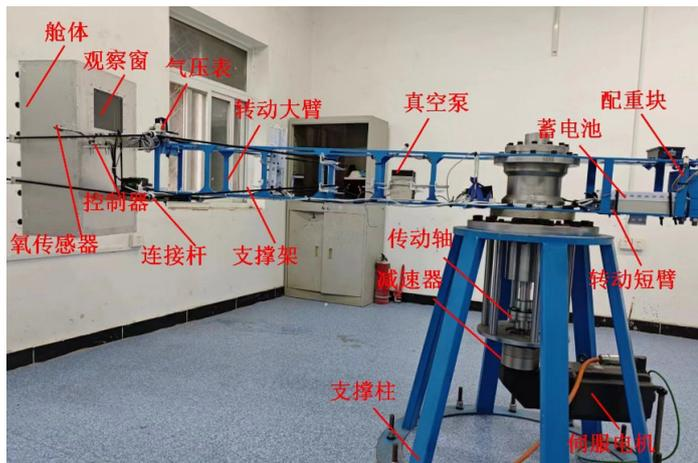
Figure 8. Photo of the low-pressure and overload integrated environment simulation platform
