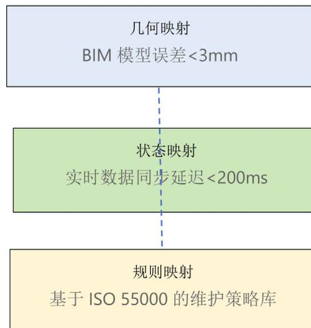
**Figure 5.** The three-layer mapping relationship for constructing the digital twin of pipelines
