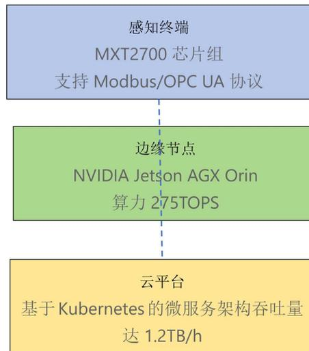
**Figure 3.** Adopting a three-tier architecture of “Edge-Device-Cloud”
