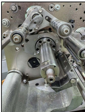
Figure 6. Physical diagram of adhesive component of adhesive tape assembly 图 6. 接装纸上胶组件实物图
